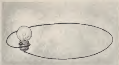
No current flows in the circuit (above left), because there is no "electron pump"—no source of power. Current flows in the circuit (above right), because the dry cell acts as electron pump.
